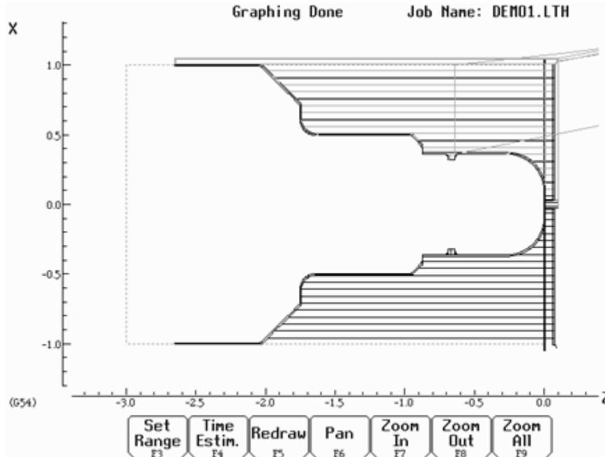
**Figure 19 - Graph of Grooving Operation – Program Line #0150**
