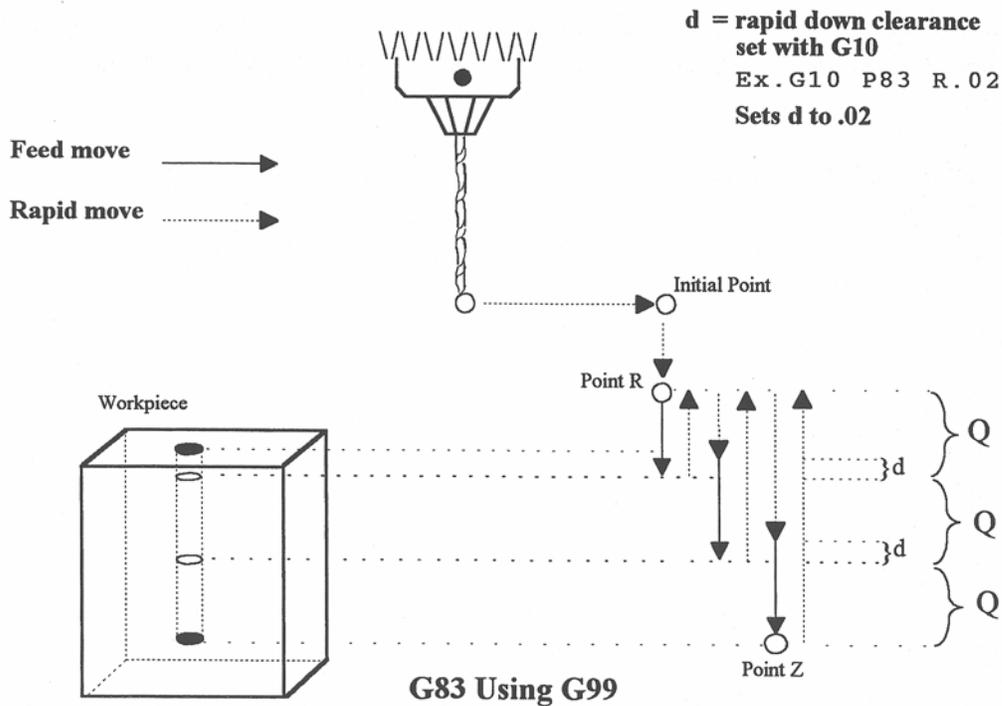
G83 is a deep hole drilling cycle. It periodically retracts the tool to the surface to clear accumulated chips, then returns to resume drilling where it left off. The retract and return are performed at the rapid rate. Because there may be chips in the bottom of the hole, the tool does not return all the way to the bottom at the rapid rate. Instead it slows to feedrate a short distance above the bottom. This clearance distance is selected by setting Parameter 83 with G10 (see example below).
