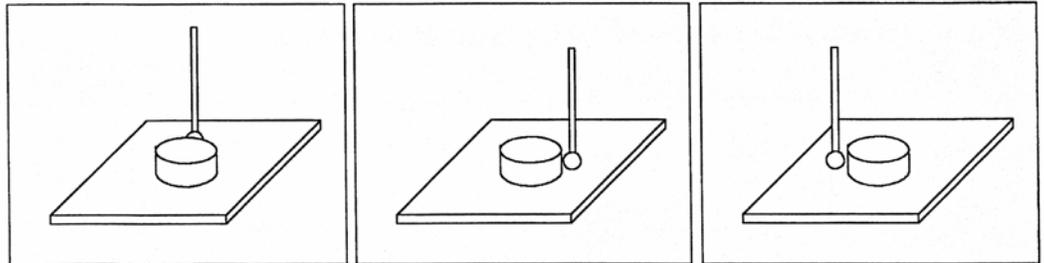
If the Z clearance you entered is too small, the probe will stop and show an error message. Correct the problem by repeating the previous steps. If the approximate diameter you entered is too small, the probe will bounce by 10 percent of its diameter across the top surface until it either finds the correct edge, the additional distance searched is equal to Parameter 16, or a travel limit is reached.
