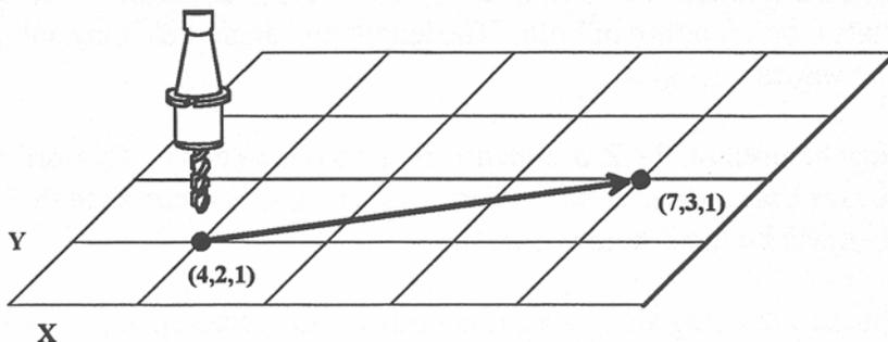
**End:** When you first access the linear mill screen, the cursor will be highlighting the first field, End X. This is the X coordinate of where the cutter will be after the linear move has been completed. Similarly, Y and Z represent the coordinates of the cutter after the linear move is completed. The angle and length fields will be computed if you choose to enter the end point of the move.
