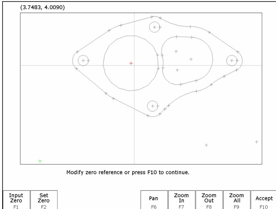
This menu allows you to change the absolute zero reference of the DXF file. The current zero reference appears as a green cross. All other points appear as gray crosses. A new zero reference may be defined by a combination the following methods:
