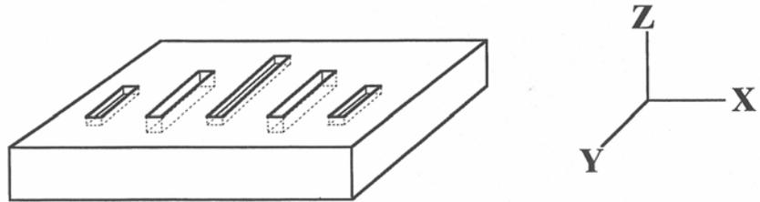
The macro variables would handle the length in the Y direction and depth in the Z direction:
