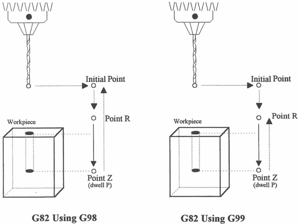
G82 is a general purpose drilling cycle similar to G81. However, G82 includes an optional dwell at the bottom of the hole before retracting the tool. This can make the depth of blind holes more accurate.
