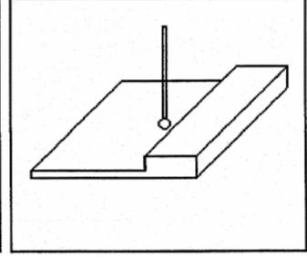
Once the probing cycle is complete, the probe will move away from the surface by the amount entered in Parameter 13 (Recovery Distance). The dimension where it found the surface will be shown on the control. Press **ESC** to return to the Set Part 0/ Position screen or digitize screen.
