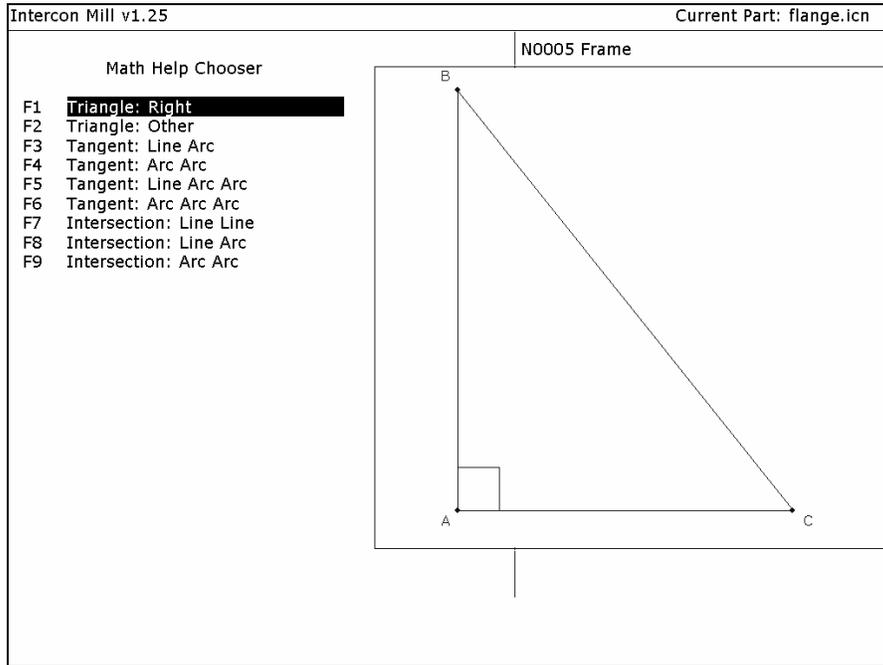
The figures on the right are a graphical representation of the highlighted solver on the left. Pressing **ENTER** key will display another menu that has various fields particular to the type of problem that is being solved. The graphic below displays the Right Triangle Calculator menu. The options that are available on the function keys are the same for every type of math help solver and perform the following operations:
