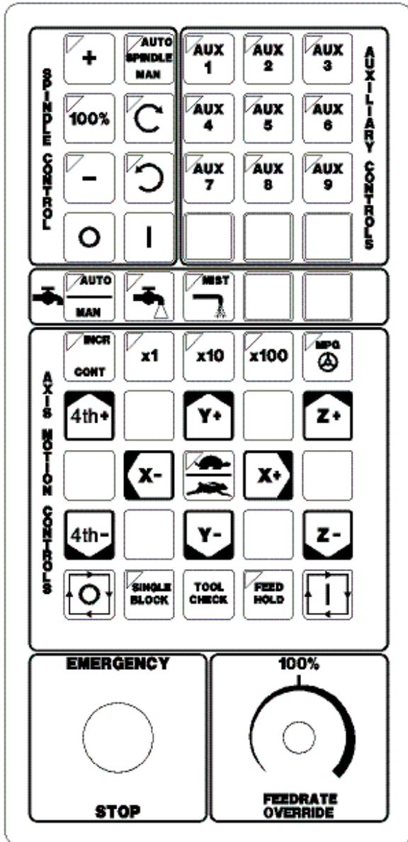
The M-Series operator panel is a sealed membrane keyboard that enables you to control various machine operations and functions. The panel contains momentary membrane switches, which are used in combination with LED indicators to indicate the status of the machine functions.
