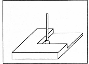
At the end of the probing cycle, the probe will be positioned above the corner at the Z clearance level entered. Press **ESC** to return to the Set Part 0/ Position screen or digitize screen.
