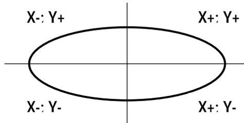
If the probe bypasses a contact point on the Y axis, it will continue moving in the X direction across the center line until it reaches the patch length limit and faults out.
