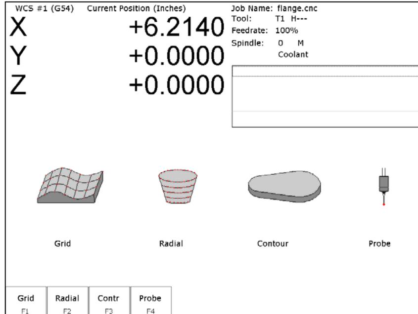
The Digitize feature of CNC10 is used to digitize a rectangular surface area (grid), an inside circular bore area (radial), or a contour. The digitizing process creates a file with M & G codes that represent the digitized surface. If the digitizing probe tip is chosen to match the milling cutter size, the digitized file can be loaded and run to produce an exact copy of the digitized part.
