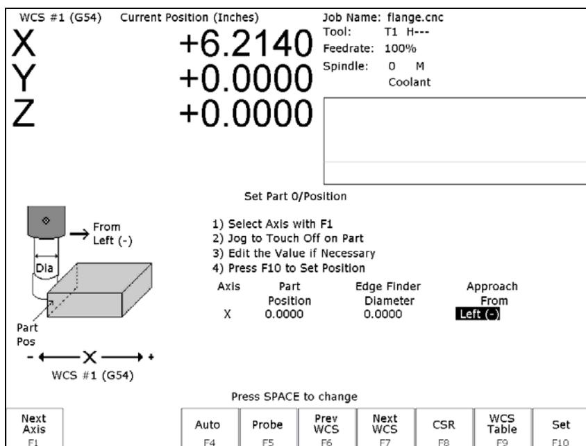
**WARNING: Before manually jogging any probe, make sure the machine Feedrate is slow (less than 10 in/min) or damage to the probe may result!**
