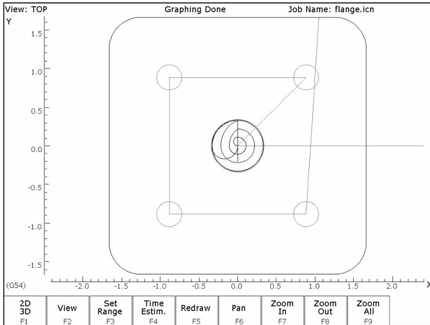
The display will consist of arcs and/or lines that make up the tool path followed. Rapid (G0) moves will appear in Red, linear (G1) and arc (G2, G3) moves will be Yellow, and compensated pass will appear in gray. Canned cycle operations (except the facing cycle) will also display a gray.
