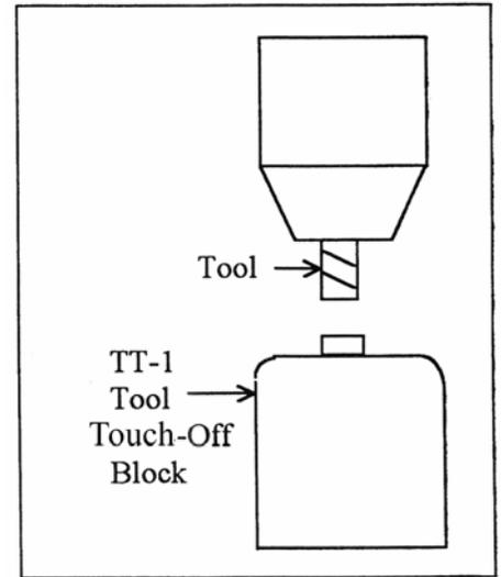
1. Load the probe into the machine.
