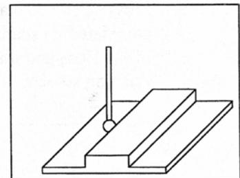
If the Z clearance you entered is too small, the probe will stop and show an error message. Correct the problem by repeating the previous steps. If the approximate width you entered is too small, the probe will bounce by 10 percent of its width across the top surface until it either finds the correct edge, the additional distance searched is equal to Parameter 16, or a travel limit is reached.
