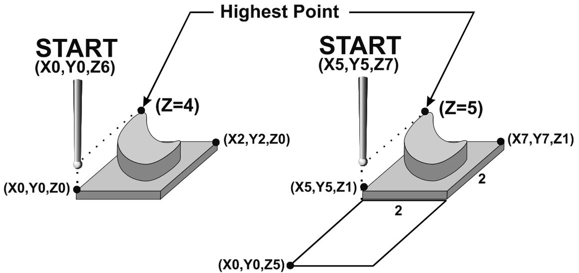
3. A good technique for calculating Z maximum depth is to touch off the lowest surface of the part to be digitized and set the part zero's Z value to Z0. Then jog the probe tip to a point higher than the highest surface of the part to be digitized. Note the displacement in the Z-axis. Again, set this Z height to Z0 and use the noted displacement for the Z maximum depth.
